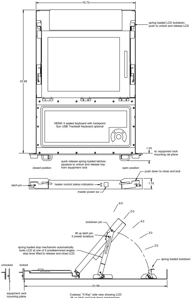
Cutaway "X-Ray" side view showing LCD lift up latch and lock-down mechanisms
