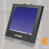
Ruggedized, sunlight readable LCD for outdoor operations. Includes waterproof speakers and VESA mount. Built-in handle and retractable stand aids portability. MIL810 compliant.
