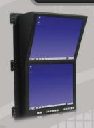
Dual 19" LCD display in hinged door configuration, mounts to front surface of IEC enclosure, freeing valuable rack space for additional equipment.
