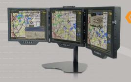
Triple 19" LCD desktop VESA mount display folds up for compact storage and portability. Multiple input and touchscreen options available.
